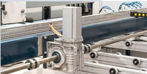
The pusher travels through precision pinions and racks. The precise positioning of the pusher is achieved by a magnetic band (no contact system). The grooved pressure beam allows the grippers to keep the panel's clamped until the final cut. The extremely fast servo-drive technology guarantees shortest cycle times.
