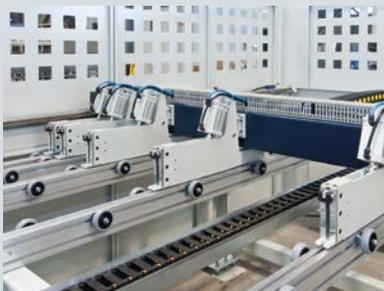
The pusher travels through precision pinions and racks. The precise positioning of the pusher is achieved by a magnetic band (no contact system). The grooved pressure beam allows the grippers to keep the panel's clamped until the final cut. The extremely fast servo-drive technology guarantees shortest cycle times.
