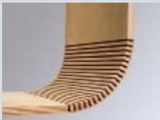
System for grooving cuts in automatic sequence
