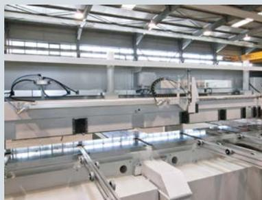
A robust torsion bar and precision rack guarantees a perfect parallelism of the pressure beam with respect to the working table. The handling of the machine becomes with a very easy and friendly control system that allows the fast implementation of cutting programs.
